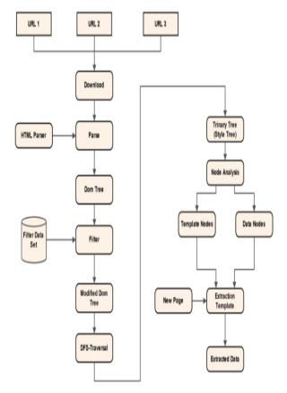
Figure Architecture of proposed system
